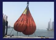
Load test of vessel's crane using load cells & waterbags
