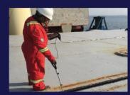
Ultrasonic testing of hatch covers to ensure water tight integrity. Loss prevention surveys.
